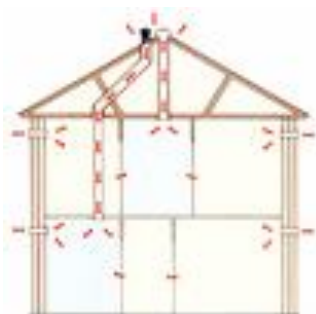
Passive ventilation System
